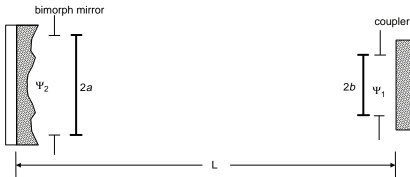
FIGURE 6.9 Schematic setup of the CW CO 2 laser with adaptive mirror.
