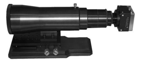
Fig. 4. Photography of our Shack-Hartmann wavefront sensor
