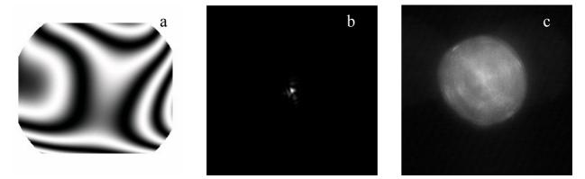
Fig. 6. Nd: YAG laser beam investigation. a – wavefront of the beam, b – calculated far field intensity distribution, c – measured far field intensity distribution
