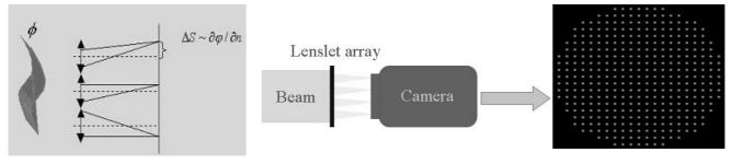
Fig. 3. Idea of Shack-Hartmann wavefront sensor
